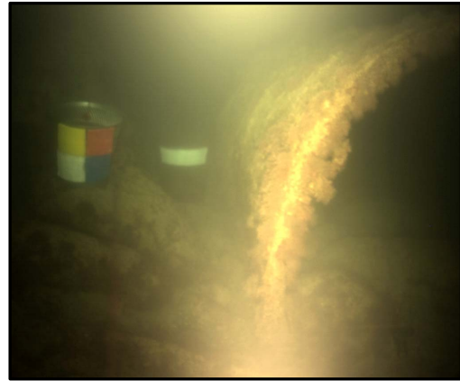
Figure 1. An underwater image taken in the Mediterranean with two artificial light sources. The backscatter greatly degrades visibility, and its nonuniformity creates dynamic range problems.
