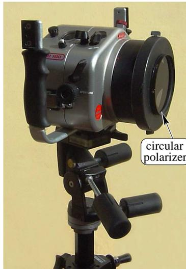
**Figure 1.** The Aqua-Polaricam mounted on a tripod.
